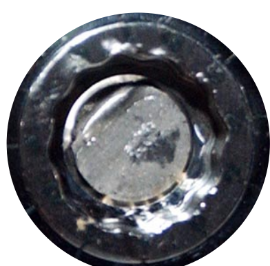
Fatigue failure c.c. modular neck.
