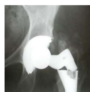
Fractured titanium SROM® stem.
