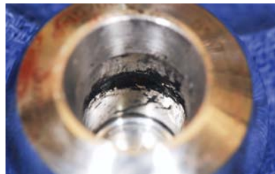
Figure 1e. Corrosion and debris within femoral head.
