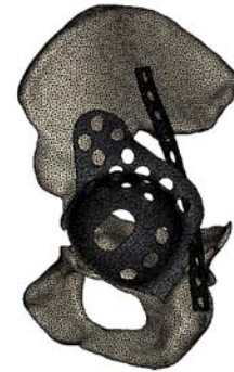
Figure 2. Position of the Burch-Schneider cage and the reinforcement plate in the large defect model
