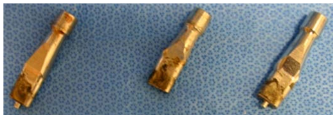
Figure 16d. Explanted Stryker ABG II Modular Necks Showing Fretting and Corrosion (Courtesy of WL. Walter)
