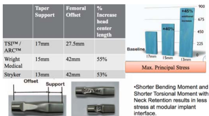
Figure 16a. Showing Modular Necks taper support engagement and percent increase in stress for engagement support.
