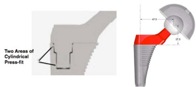
Figure 20. Dual-Press Modular Junction (Omni, East Taunton, MA) Illustration Showing two areas of press fit allowing proximal shoulder to sit flush with stem body.
