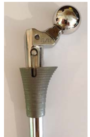
Figure 27a. 1984 Polished S-Rom 125° Stem with Proximal Modular Sleeve that engaged a de-rotational locking pin in the stem. (Stem Ti-alloy, Ti-alloy Modular Sleeve & Co-Cr-Mo Modular Head. (JMPC, Stanford, CT) (Courtesy of JISRF)
