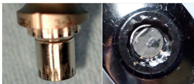
Figure 22a. Pictures showing a fatigue failures in explanted OTI Co-Cr-Mo modular neck and close up of broken neck within the stem cone body. Stem, neck and head are Co-Cr-Mo. (Courtesy of JISRF)
