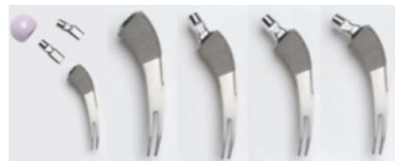
Figure 6. Picture of ARC™ Stem Showing Modular Necks in various positions (Valgus, Neutral & Versus) Co-Cr-Mo, Ceramic Head Taper 12/14, Titanium Alloy Stem with Proximal Porous Pure Titanium Plasma Spray Coating with a Surface Layer of HA Coating. (Courtesy JISRF Archives)
