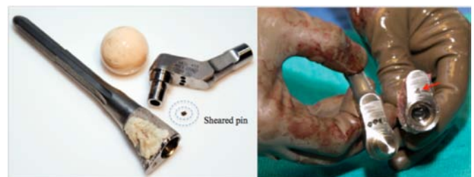
Figure 21b. Explanted Apex Modular Stem (Dual Press Modular Junction, Omni, East Taunton, MA) showing sheared de-rotation pin and fretting abrasion wear. No signs of corrosion. (Courtesy of Keggi)
