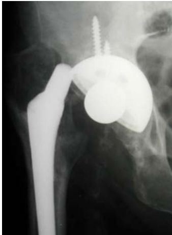
Figure 12a. Detachment of modular head can damage stem trunnion. (Courtesy of J. Keggi)
