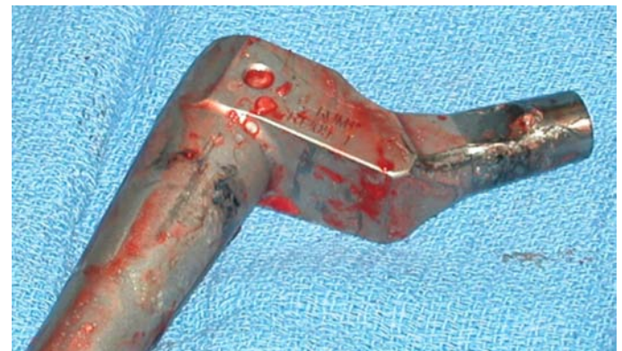
Figure 26. Explanted S-Rom Stem showing surfaces scarring (metal transfer) on the proximal stem under the modular sleeve and under the shoulder of the stem. This demonstrates micro-movement between the modular junction. (Courtesy of JISRF)
