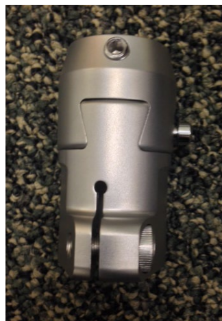
Figure 13: Posterior view of coupler.
