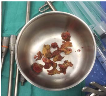
Figure 7. Tissue and bone debris showing slight staining from corrosion action of modular neck-stem taper. Courtesy of B. Vaughn
