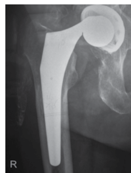
Image 11: Patient 4: Presenting anteroposterior radiograph of the dissociated head-neck junction of the right THA.
