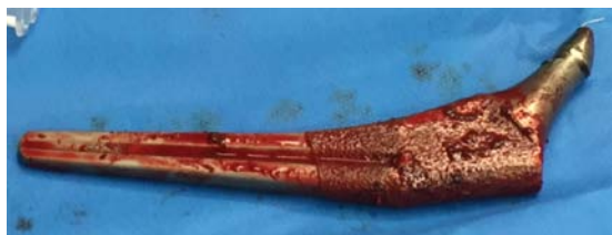
Image 5: Patient 1: Retrieved femoral stem showing marked corrosion of the neck taper.
