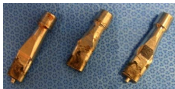
Figure 3. Retrieval of taper corrosion with dissimilar metals—cobalt-chrome alloy modular neck on titanium stem. (Courtesy WL Walter)
