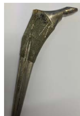
Image 10: Patient 3: Retrieved femoral stem with marked neck taper corrosion and inferior notching.
