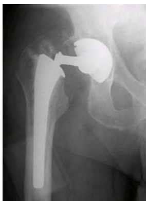
Figure 2. Fatigue Failure of C.C. modular neck used with a c.c. Cemented stem.(R-120™ Encore Orthopaedics) (Courtesy JISRF & H.U. Cameron)
