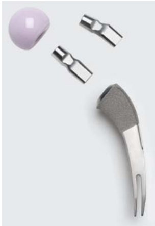
Figure 6. Omni ARC™ Stem (Omni, Raynham MA) Titanium Alloy Stem with HA and pure titanium plasma spray coating with a c.c. Modular neck.
