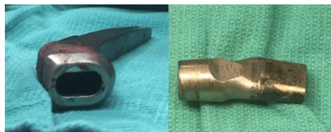
Figure 5. Explanted ARC stem 5 years post-op (Omni, Raynham MA.) Courtesy of B. Vaughn
