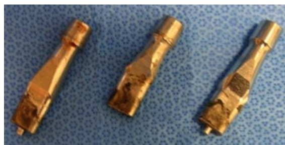
Figure 3. Retrieval of taper corrosion with dissimilar metals—cobalt-chrome alloy modular neck on titanium stem. (Courtesy WL Walter)
