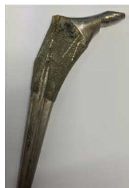
Image 10: Patient 3: Retrieved femoral stem with marked neck taper corrosion and inferior notching.
