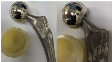
Image 8: Patient 2: Retrieved femoral stem and acetabular liner with instability evident and dissociation of the head-neck junction.
