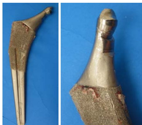
Image 12a and 12b: Patient 4: Retrieved femoral stem prosthesis with taper corrosion evident and inferior neck notching.
