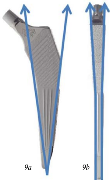
Figure 9 – Photograph of implant showing; 9a - AP view showing Design features; 9b - Lateral view showing design features
