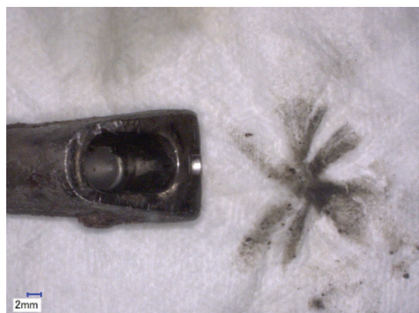
FIGURE 14-5. Retrieval of taper corrosion with dissimilar metals—cobalt-chrome alloy modular neck on titanium stem. (Courtesy Dartmouth Biomedical Engineering Center.)
