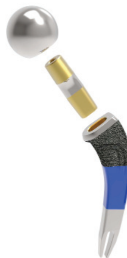
FIGURE 14-7. Rendering of modular cobalt-chrome alloy neck with a nitriding coating (gold) of the distal taper engagement with a titanium alloy stem. Providing a reduction of corrosive galvanic reaction with dissimilar metallic alloys. (Courtesy Chris Burgess, Signature Orthopaedics Ltd.)
