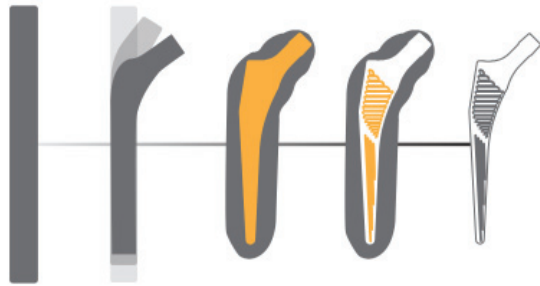
FIGURE 14-1. Hip stem forging steps. (Courtesy Signature Orthopaedics, Ltd.)
