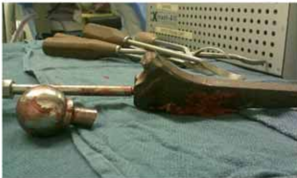
Example of a fractured Zweymüller
