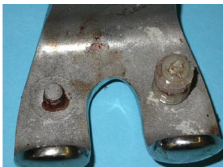
Example of HA coated knee with severe 3 body wear.
