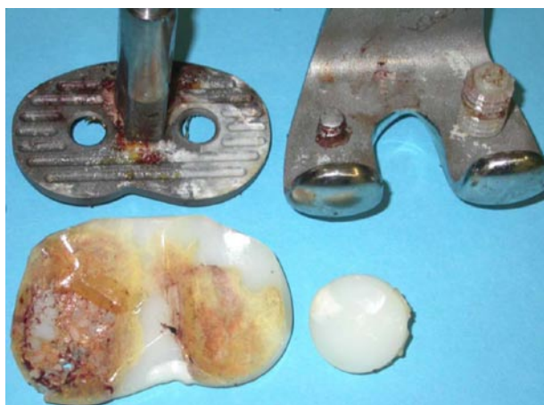
Example of HA coated knee with severe 3 body wear.
