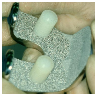
Black staining is caused by metal debris.
