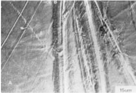
Figure 48 Example of increased wear of bearing surface.
