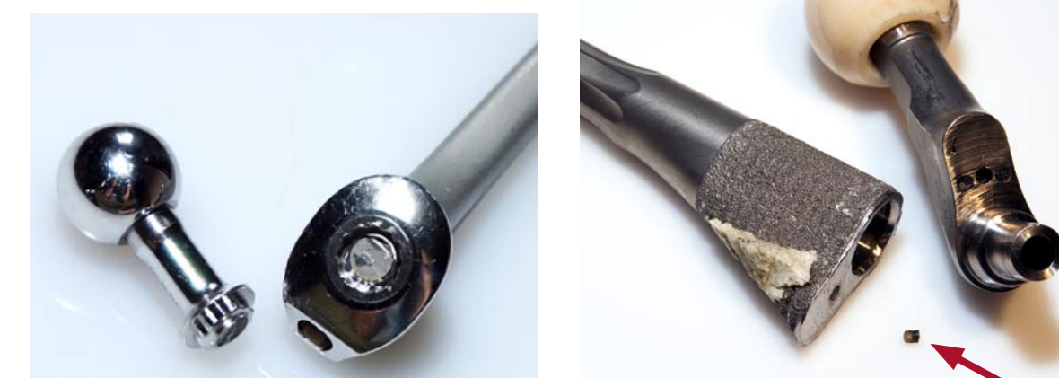
Figure A. Fractured neck.
