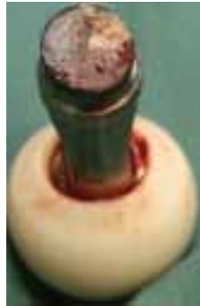
Surface damage to a head/neck taper
