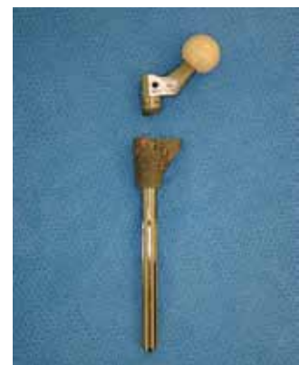
Example of a fatigue failure in a young 37 yo male 85kg / failed at 4 years (W. Walter)
