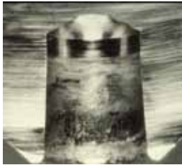
Surface damage to a head/neck taper
