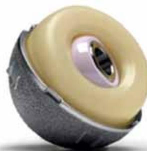
Figure 1 - Picture of dual articulation hip bearing concept. In this example, a UHMWPE head is articulating with an all-metal porous coated acetabular cup. Within the polyethylene head is enclosed an inner ceramic ball that is assembled ex-vivo at the time of surgery. Courtesy Biomet, Inc. Warsaw, IN..
