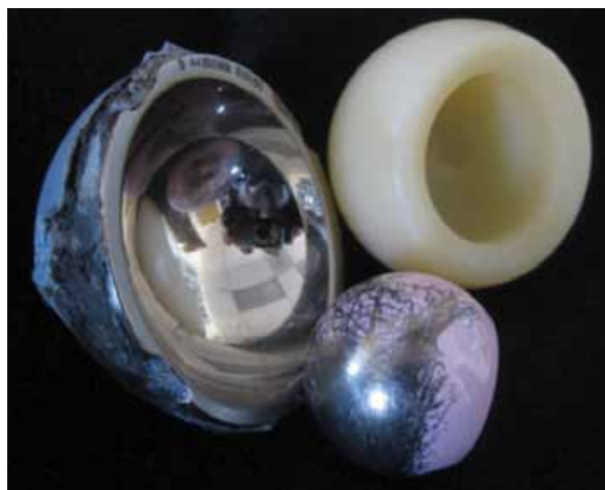
Figure 7 - Retrieved dual articulation bearing. Multiple metal smears are seen on the ceramic head which was articulating upon the metal cup.
