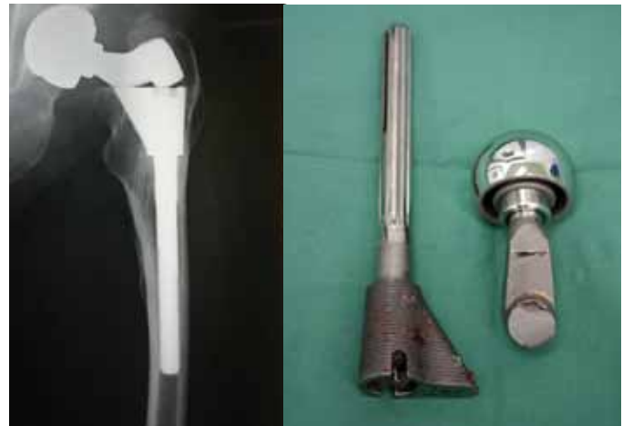
Example of a fatigue failure in a young 37 yo male 85kg / failed at 4 years (W. Walter)
