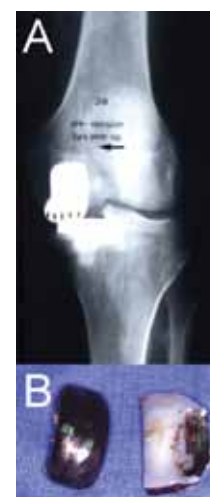
Fig. 2 Wrong component sizing or positioning may lead to edge loading (A) resulting in increased wear and implant failure (B).
