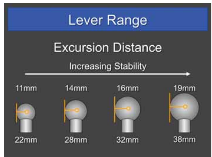
Fig. 7. Photograph demonstrating the effect of increasing head to neck ratio. In this example, head diameter increases while neck diameter remains the same. Hip range improves in proportion to the increase in head to neck ratio. Although the large diameter head may not dislocate, it is susceptible to repetitive levering. Repetitive levering scratches the head at the edge of the acetabular rim.
