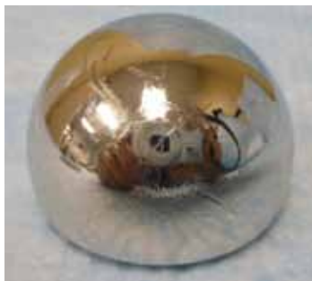
Fig. 3. Photograph of retrieved head. Note the long scratches from the reduction maneuver. Also note at the base of the ball, the multiple metal pits. The pitting phenomenon is best described as an asteroid impaction zone. We suspect this area was damaged by free carbide fragments that were crushed between the bearing surfaces.
