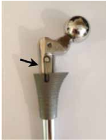
S-Rom Grooved Style had a polished stem with a vertical groove & locking pin. The groove acted as a funnel for migration of poly debris causing distal bone lysis.
