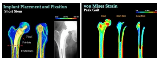
The FEA analysis demonstrates better strain patterns compared to fully porous coated straight stem design.
