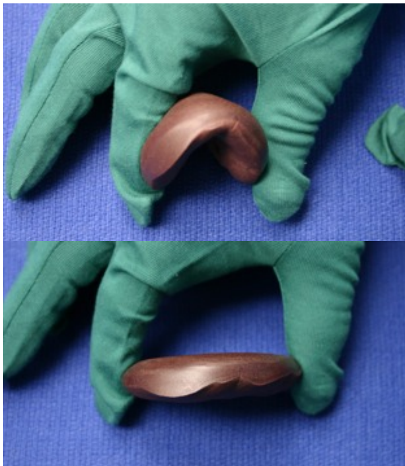
Fig 1b. Same sample of Palacos® R-rifampin showing how the cement puck easily bends without breaking. Once bending force is released, the specimen returns to its resting flat state.
