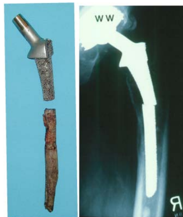
Distal stem fixation can also result in a cantilever effect resulting in stem failure.
