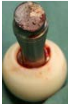
Surface damage to a head/neck taper
