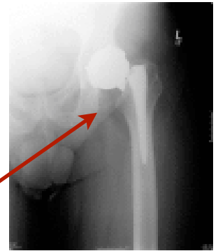
Fx. Profemur Z stem/neck 4 yrs post-op Wright et al.
