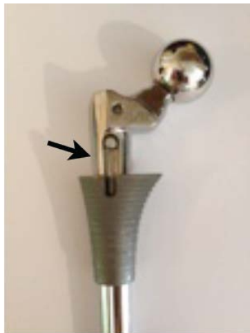
Example of a fatigue failure in a young 37 yo male 85kg / failed at 4 years (W. Walter)
