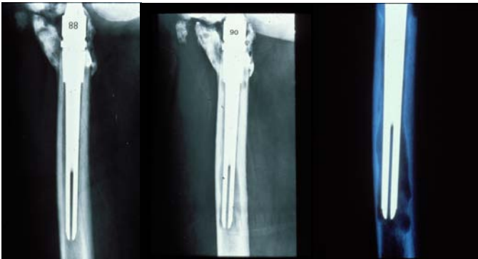
S-Rom grooved style stem progressive osteolysis C. Engh. Groove in the stem allowed migration of debris. Resulting in a stem design change.
