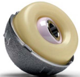
Figure 1 - Picture of dual articulation hip bearing concept. In this example, a UHMWPE head is articulating with an all-metal porous coated acetabular cup. Within the polyethylene head is enclosed an inner ceramic ball that is assembled ex-vivo at the time of surgery. Courtesy Biomet, Inc. Warsaw, IN..
