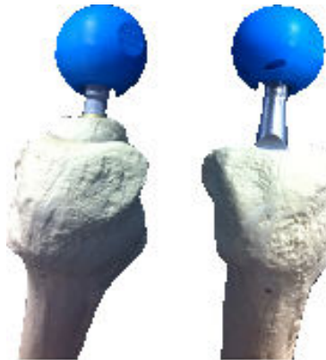
Figure 7. Varus /Valgus turning moment in neck retention vs. conventional neck resection
